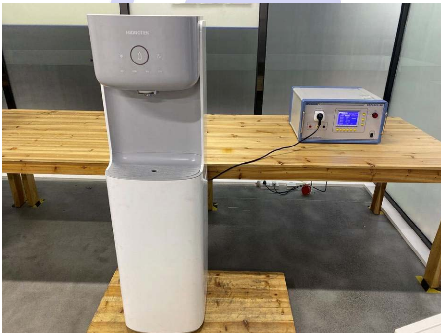
16.8.Photo of Voltage Dips and Interruption Immunity Test
