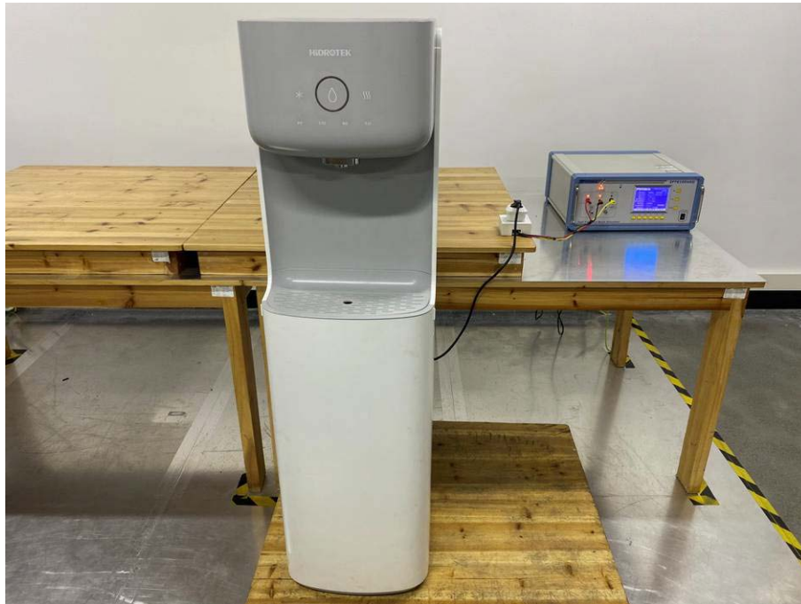
16.5.Photo of Electrical Fast Transient /Burst Test
