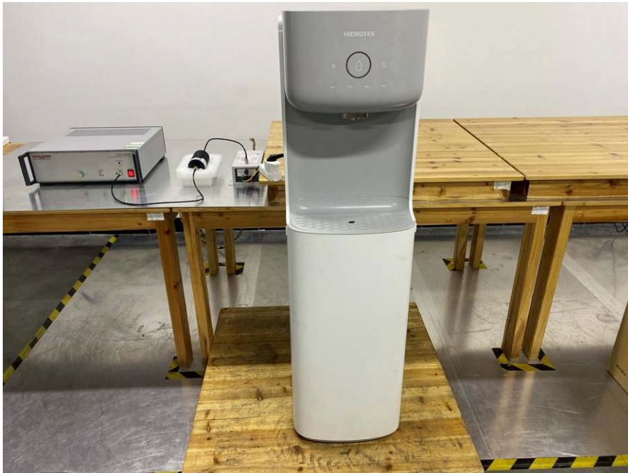
16.7.Photo of Injected Currents Susceptibility Test
